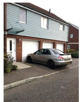
An example of poor design, resulting in footway obstruction due to an overhanging parked vehicle.
